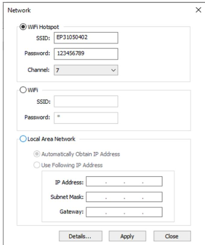
**3.1.8, Set up multiple ezPosters in the same network:** There are 2 ways to allow multiple devices listed in the device list under one network.
